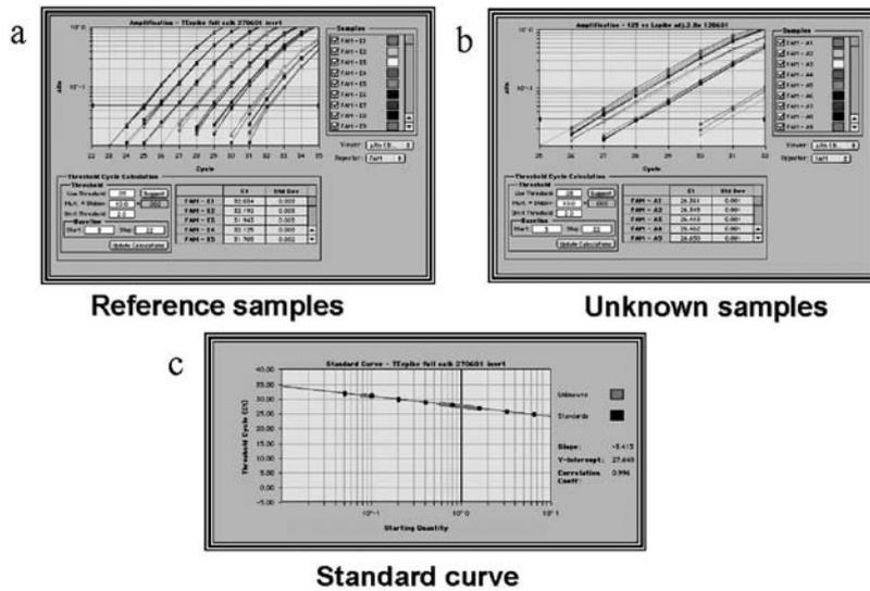
**Figure 6.** Example of GMO quantification by real-time PCR. Both standard (a) and unknown samples (b) are analysed within the same experiment; the Ct values obtained from the amplification of the standards (c - black dots) are used to build the regression standard curve on which Ct values of unknown samples are plotted (c – gray dots)
