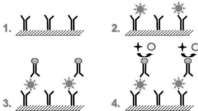
**Figure 7.** Fundamental steps in the 'sandwich' ELISA test: 1) Specific 'capture' antibodies are lined at the bottom of each well of the microtiter plate; 2) upon addition of a positive sample, the 'capture' antibody binds the antigen of the target protein; 3) the 'detector' antibody, conjugated to an enzyme, is added forming a "sandwich" complex; 4) enzymatic development of a detectable signal upon addition of appropriate substrate
